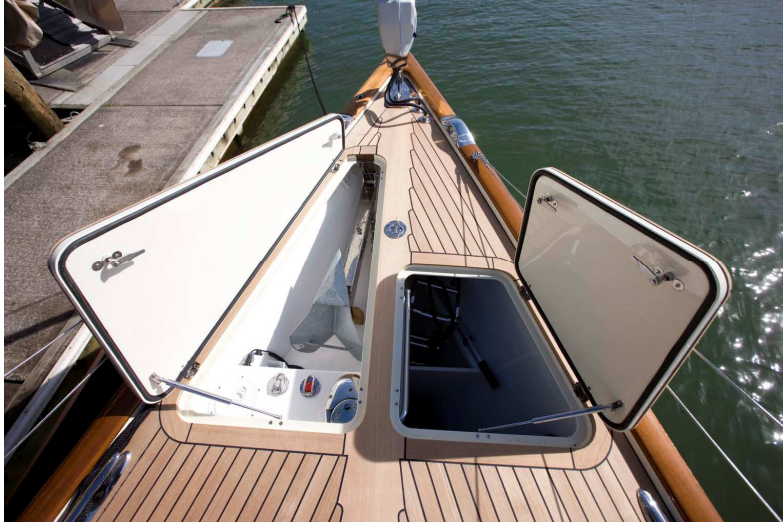
Anchor swing out system to port, chain locker and large storage to stbd.
