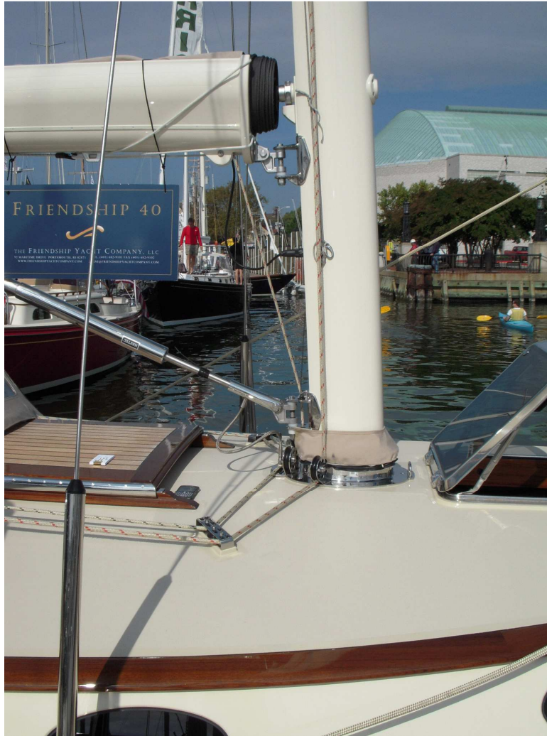
Stainless steel hydraulic vang, in-boom main furler, and mast collar with custom built-in stainless steel turning blocks.
