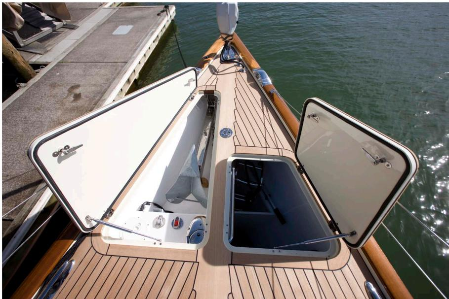
The foredeck houses two flush lockers – to port is the swing out anchor system with *Lewmar* electric windlass and saltwater wash down, to starboard is the chain locker with storage for swim ladder and dinghy outboard motor. The custom chocks in the cap rail are larger on the foredeck than those aft to accommodate large mooring lines, and the cleats are flush to the deck when not in use. On centerline is an additional, extra strength pop-up pad eye for hurricane tie down.
