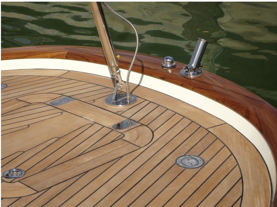
Aft deck – custom flag socket for dinghy towing, stainless steel hydraulic backstay, and flush plate for fresh water hot/cold deck shower
